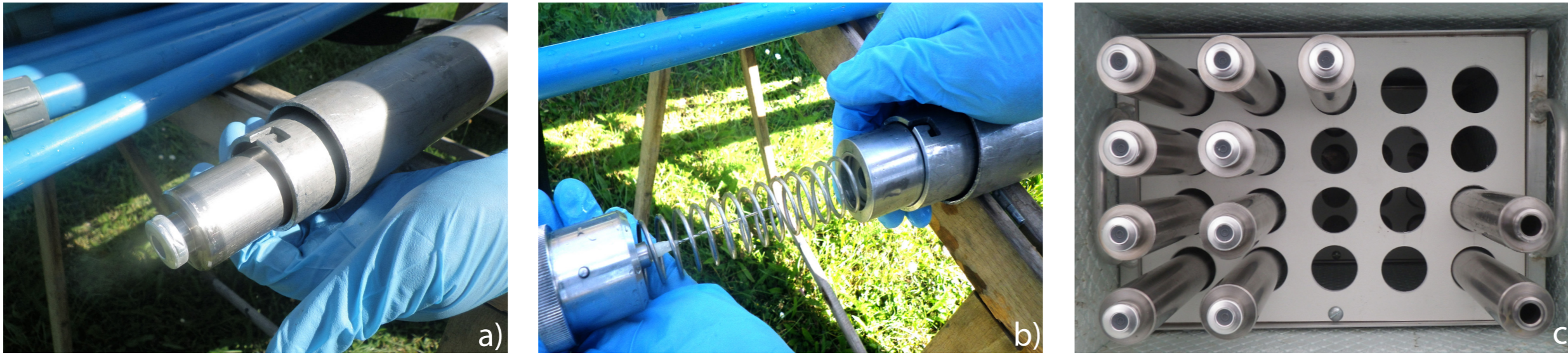
The enhanced gastight, sterilizable sampling system. a) Removal of a sample vessel from the gastight sampling system b) Close-up of the inner workings of the gastight sampling system c) Cooling box for transport of the sampling vessels
